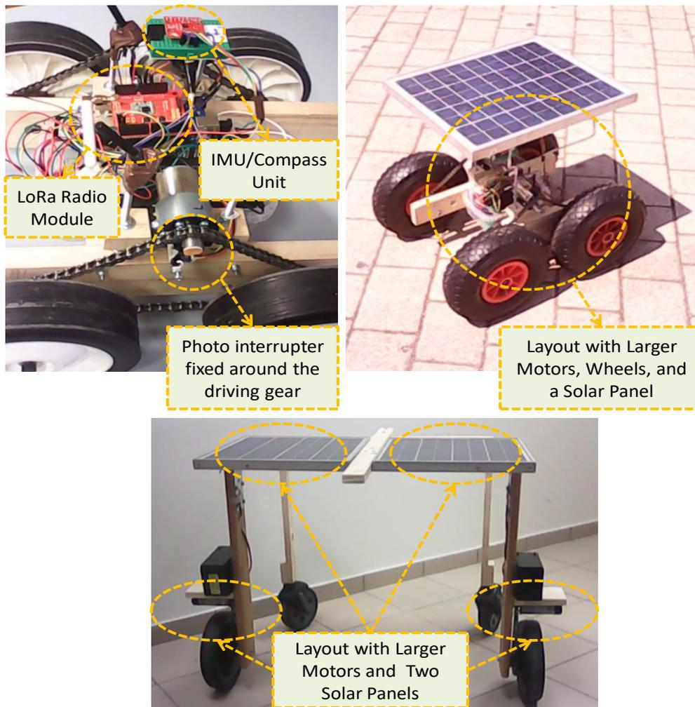
**Figure 2. Enhancements involving feedback mechanism for DC motors, IMU/Compass unit and LoRa shields for Arduino (top left). Further enhancements involving solar panel assistance and bigger motors and wheels (top right and bottom)**
