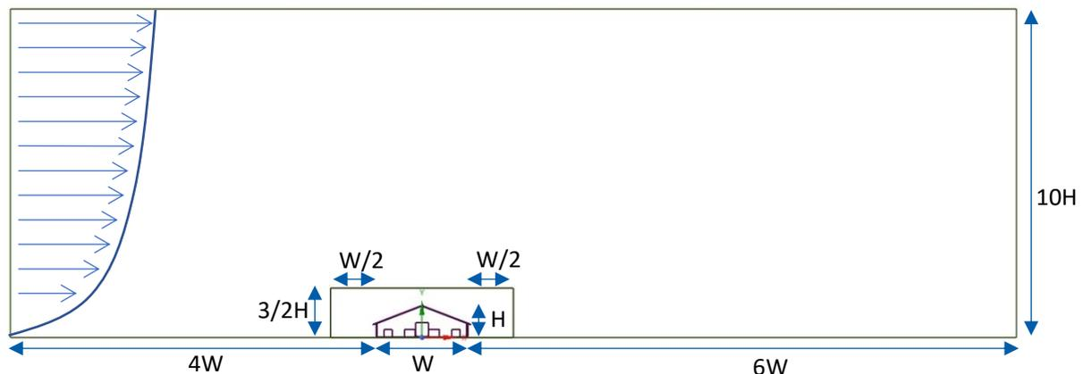
Figure 1. Dimensions of the numerical domain
