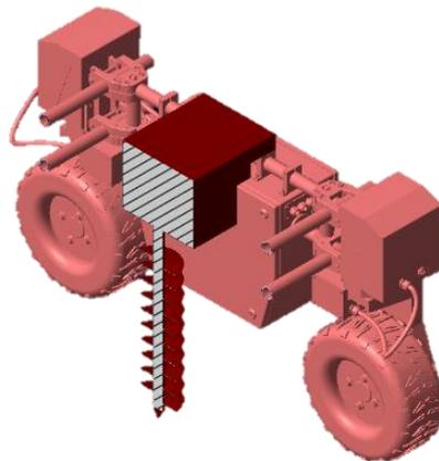
Figure 2. Section view of auger on UGV
