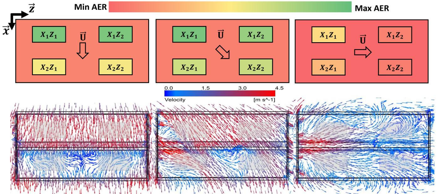
**Figure 4. Up: AER of the whole barn  $L/W=2$  and the AOZs for different incident velocity angles (from left to right:  $0^\circ$ ,  $45^\circ$ ,  $90^\circ$ ), down: corresponding velocity vector field at the middle of AOZ height; velocity magnitude 5 m/s.**
