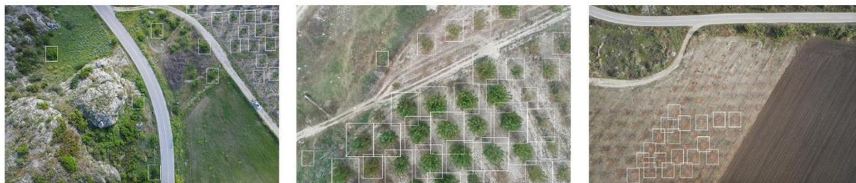
**Figure 3. Trees identified by the developed system for the image acquired during (a) May, (b) November and (c) December**
